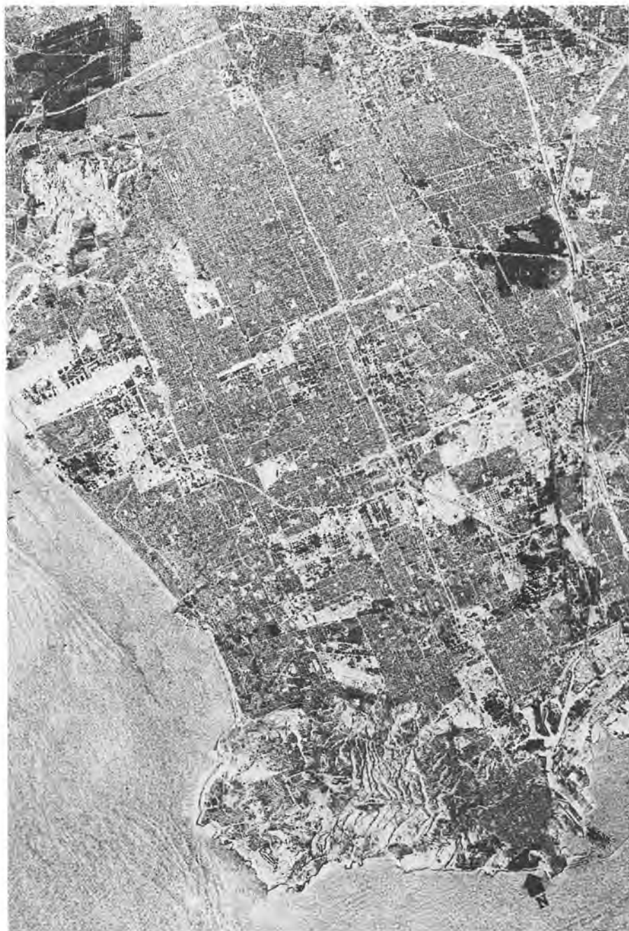
Figure 15.4. A synthetic aperture radar image of Los Angeles, California, taken from the US Seasat 1 satellite from an altitude of about 700 km at about 2030 hours local time. A considerable amount of detail can be clearly seen
