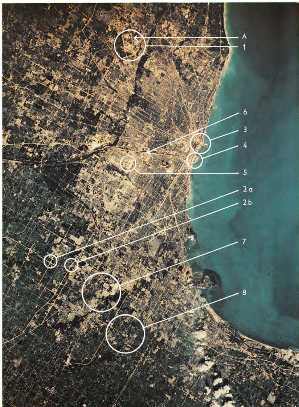
Plate 1. Chicago area photographed from the Skylab satellite at a height of about 440 km showing how clearly the O'Hare International Airport and its extensive runways (1) can be seen.
