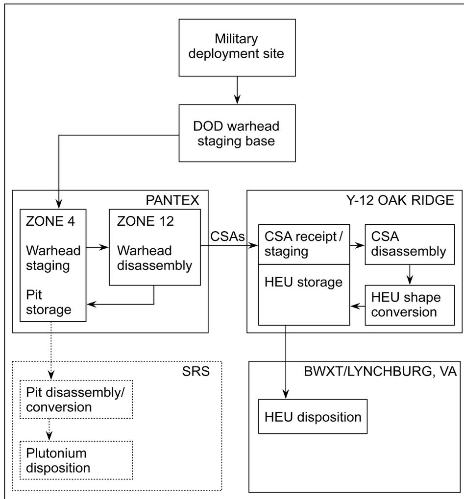
**Figure 9.2.** Warhead dismantlement in the USA
