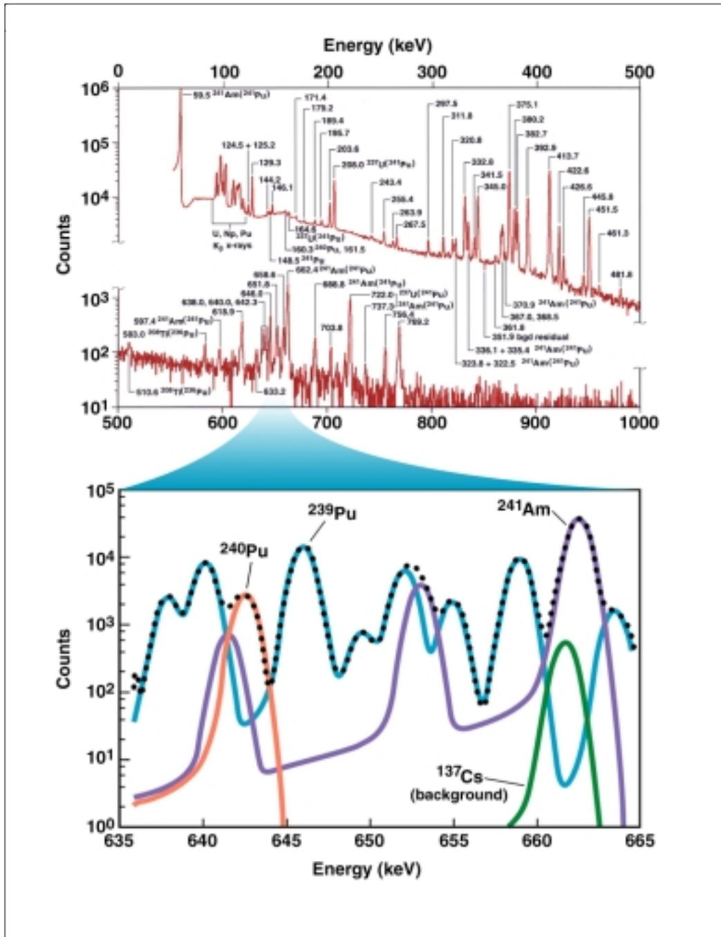
**Figure 8.1.** Measurements of the gamma-ray spectrum of plutonium
